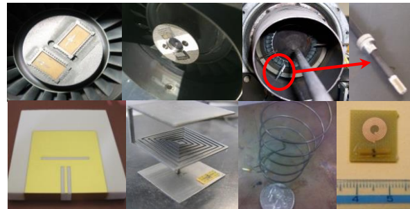
Attachment on rotating and static components
