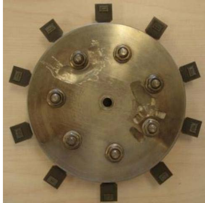
Figure 11: SAW sensors attached to test disk
